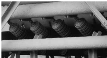
Fig. 8 - Suspended set for impact troughing set with three or five plain rollers or with shock absorbing rings
